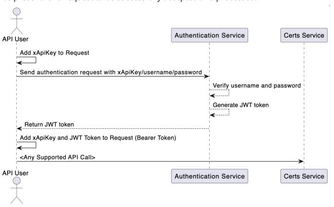
The diagram illustrates the usage flow encompassing various components engaged in the authentication process. Initially, the API user provides their username, password, and API Key (x-api-key) within a REST request to the authentication service, which then authenticates the user's credentials and generates a JWT as a response. In the subsequent
